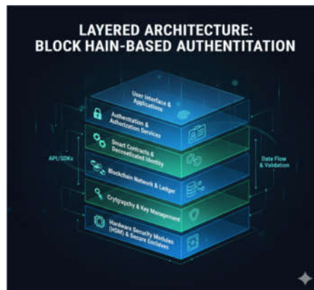
Fig. 1: Layered architecture of blockchain-based authentication system.
